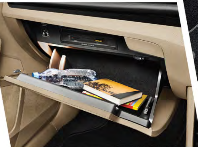
The storage compartment in the dashboard on the front passenger side can also be cooled, when the air conditioning is on.
